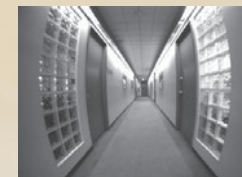
Raw Image This image shows the lens distortion for a wide angle lens.
